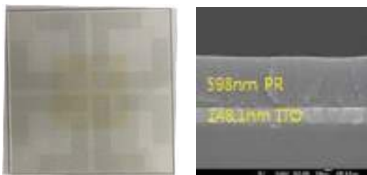
Fig. 1 Pattern on the ITO-glass and sectional view
